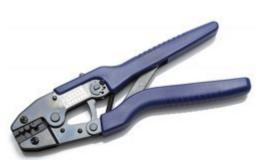
For crimping of insulated & non-insulated cordend terminals from 0.5mm to 10mm/sq. Meets the compression ratio requirements of BSEN 60999 & BSEN60998.
