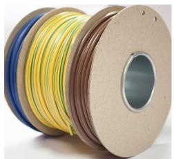
MATERIAL: CONTINUOUS TEMPERATURE: INSULATION RESISTANCE: DIELECTRIC STRENGTH: TENSILE STRENGTH: ELONGATION AT BREAK: HARDNESS: FLAMMABILITY: General Purpose PVC -20°C to 70°C 10<sup>10</sup> Ohm/cm 20 kV/mm 15MPa 220% BSS20-30 Self-Extinguishing in 30 seconds
