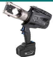
The next generation of Cembre cordless hydraulic tools represents a significantly advantageous evolution from current models. Born of the renowned B135-UC type crimping tool, first into the market is the 132kN B1350-UC, suitable for a wide range of connectors up to 400 sqmm using die sets common to the Cembre 130kN tooling range.
