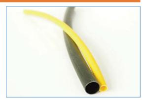
The largest size which will recover snugly over the component to be covered should be ordered. The wall thickness of the tubing will be less than specified if recovery is restricted during shrinkage.O ther lengths, sizes and non-standard colours may be available subject to special orders.
